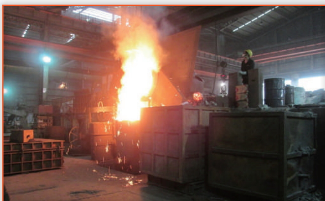
2 | 中週波熔解電爐 ( 5T ) x 2台 Five-ton Medium Frequency Induction Furnace x 2 sets
