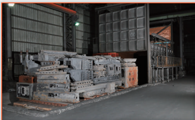
3 | 雙門雙台車式退火爐 ( 9m×4m×4m ) x 1台 Double Door, Double Trolley Annealing Furnace ( 9 m x 4 m x 4 m ) x 1 set
