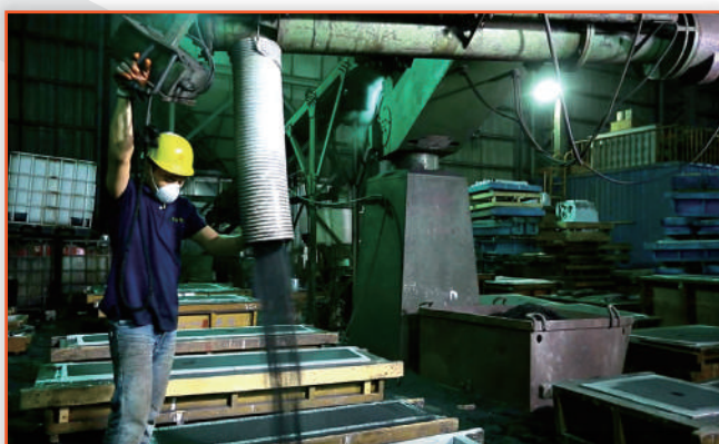
1 | 混練機 ( 10T/H ) x 6台 Furan No-bake Molding Lines (10 ton/h) x 6 sets
