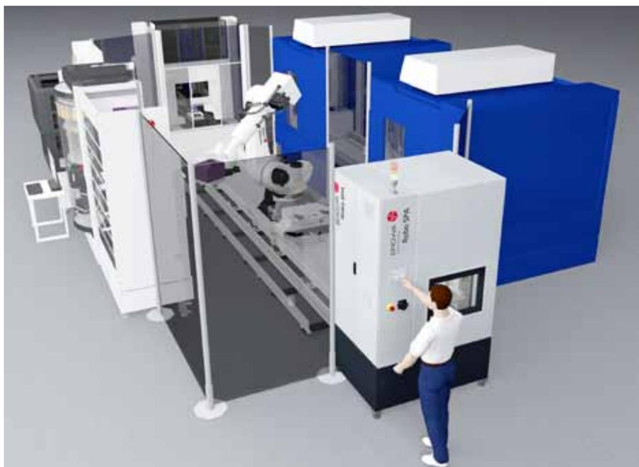
The compact cleaning station is the key to cross-process automation. The workpieces are cleaned before they are transferred from the milling stage to quality measuring or to eroding to ensure the subsequent process.
