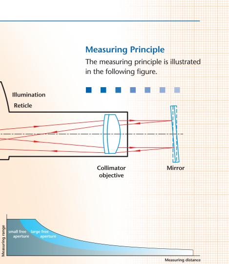
distance between autocollimator and reflector due to vignetting. This effect depends on the focal length and free aperture of the autocollimator. Since the vignetting affects the accuracy, as well, we recommend to use the **ELCOMAT direct** autocollimators only up to the maximum measuring distance given in the overview table on the back of the catalogue.
