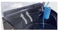
**OPTIONAL EXHAUSTION OPENING:** Exhaustion of up to 90% of the arising emission of aerosol in the back working area. For increased product and operator's safety.
