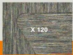
30° interior / exterior corner control Wire diameter 0.2mm
