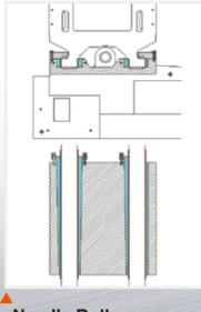
Needle Roller Bearings Slideways
