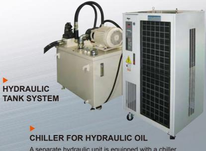
A separate hydraulic unit is equipped with a chiller system to avoid transference of heat and vibration from hydraulic system to the machine.
