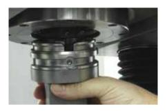
Punches and dies can be clamped and replaced quickly and precisely. The repeatability is < 0.002 mm.
