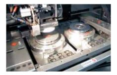
**Wire-EDM**Continuous contours in dies and punches are machined on the WEDM machine.
