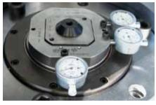
The chucks are precisely aligned to each other with the help of a specially designed alignment set. There is no need for further adjustments.
