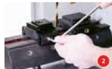
Position and fasten the clamping element Securely clamp the workpiece. based on the size of the workpiece.
