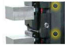
For setups with recurring workpieces: single part recognition with identification chip and the EROWA Manufacturing Control process control system.
