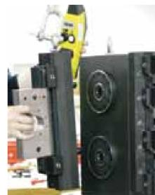
Heavy fixtures can be handled easily with a crane. The CleverClamp base rails have holes on both sides to attach eye bolts.
