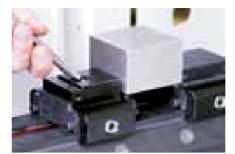
By setting up and adjusting the workpieces outside the machine, time is optimally used and cost is reduced.
