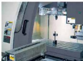
All machines are measured by laser equipment to attain high positioning and repeated accuracy with pitch and backlash compensation.
