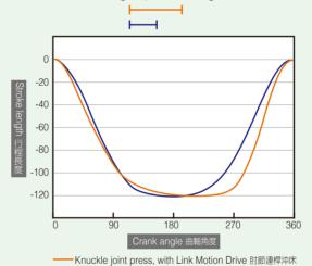
With an innovative hybrid drive mechanism of combining knuckle joint and link motion to achieve an optimal slide motion curve for precision progressive cold forging and near net shaping 以連桿機構推動肘節,具最佳滑塊運動曲線, 適用於連續沖鍛成型加工。
