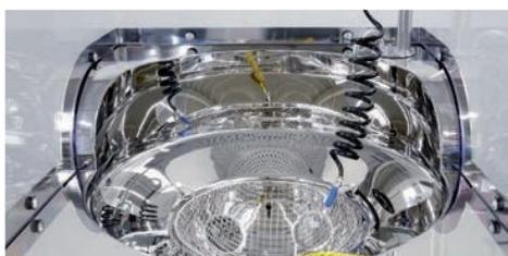
**ANALYSIS AREA** (500 mm) with round basin (300 mm) with polished stainless steel interior. Components from 3-5 kg can be tested with the help of a parts holder. Different extraction options: rins/spray, flood, ultrasound.
