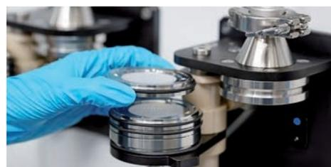
**THE USER-FRIENDLY**, lifting and tilting membrane holder includes three individual cascade rings with tweezer leads for safe and simple membrane fitting and removal of  $\varnothing$  47 mm membrane filters.
