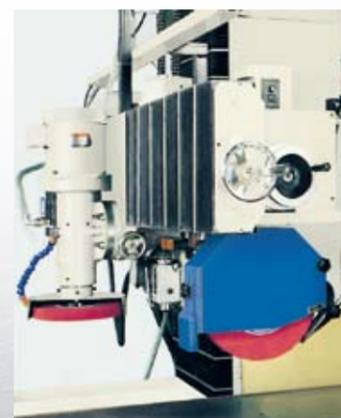
▲ Vertical Spindle Grinding Equipment (Optional Accessories)
