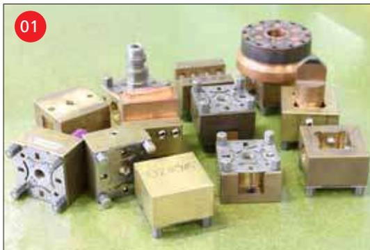
Check the general condition of the electrode holders for damage on the chuck body (thread, contact surfaces for blanks), the supporting feet and the centering plates (worn-out punch holes).
