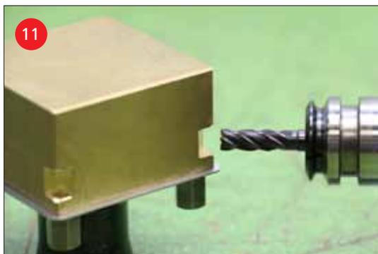
If the retrofitted ITS 50 Holders C are loaded by means of a Robot, then the gripper slot must now be reworked.
