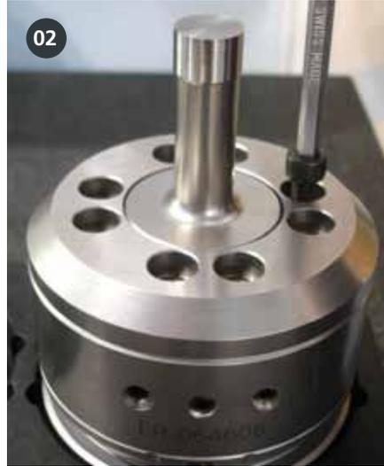
02 The punch can thus be mounted and clamped in the adaptation pallet.
