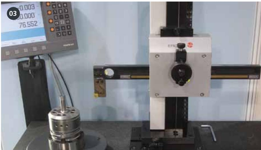
03 The pallet is clamped pneumatically on the alignment device –
