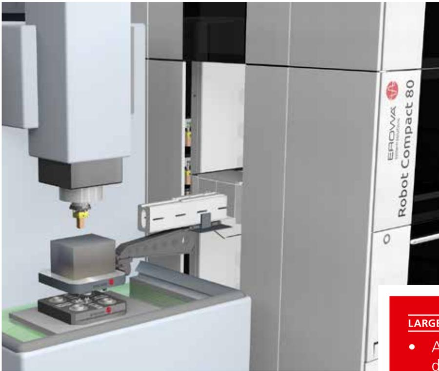
Even large UPC 320 pallets of up to 80 kg transfer weight are loaded accurately onto the machine.
