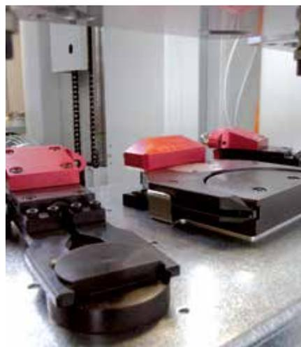
The EROWA Robot Compact 80 automatically changes the grippers according to the pallet size.
