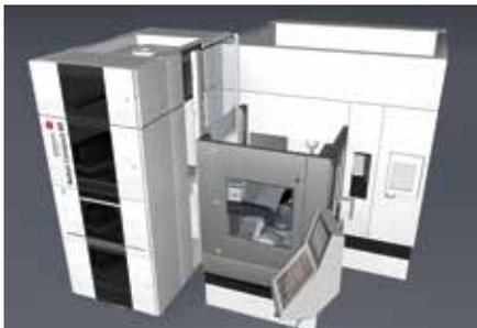
EROWA Robot Compact 80 loads a 5-axis machining center from the side.
