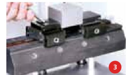
Securely clamp the workpiece.
