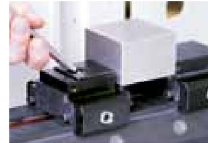
By setting up and adjusting the workpieces outside the machine, time is optimally used and cost is reduced.
